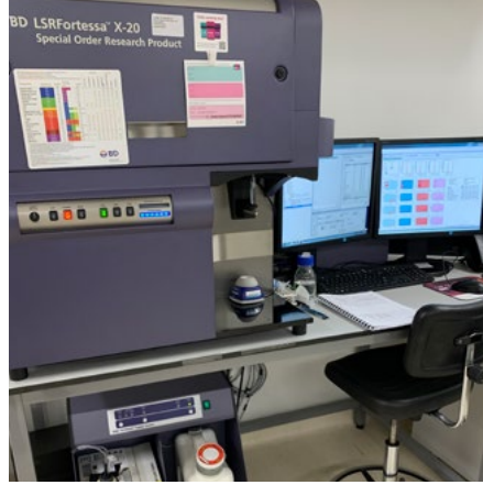
The BD LSRFortessa X-20™ Analyser can quickly measure cell-level detail with statistical significance.
