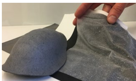
Fabrican Ltd sprayable fabrics for face masks: white, containing antimicrobial cationic surfactant and carbon black; black, containing activated charcoal; grey, with activated charcoal; transparent, to facilitate communication, containing antimicrobial surfactant.
